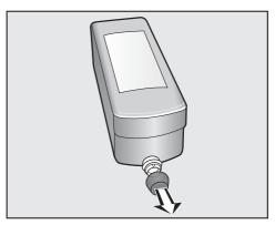
■ Remove the cap from the cartridge.
